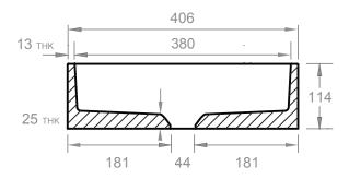
mudd works to tolerances of +/- 5mm. SCALE 1:8 rev. 01/25
