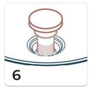
Slide drain into place and add a **generous** amount of silicone to drain seal or nut underneath. Secure drain by hand tightening no more than a 1/8" turn. **Do not overtighten.**
