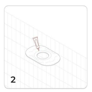
Install wall finishing over timber frame and apply silicone directly onto bracket surface.
