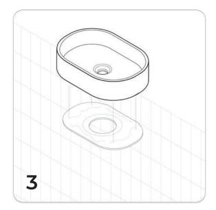
Carefully lower and place basin onto siliconed bracket firmly. Remove any excess silicone on the underside of the basin with a microfiber cloth.
