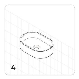
Allow silicone to sit and dry for 12 hours prior to installing plumbing fixtures.
