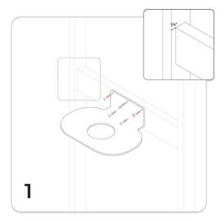
Install 2x6 timber backing, set back approx. 1/4" from stud face, at desired height. Screw in bracket to timber frame and secure in place.
