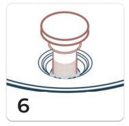
Slide drain into place and add a **generous** amount of silicone to drain seal or nut underneath. Secure drain by hand tightening no more than a 1/8" turn. **Do not overtighten.**
