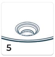
Run a **generous** amount of clear silicone around the drain rim. It is important that the silicone overflows when drain is placed through the opening.
