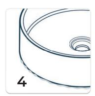
Run a bead of clear silicone to fill the gap between the basin and the surface. Smooth silicone off to a neat finish. Ensure edge is fully water-proofed. Allow silicone to sit and dry for 12 hours prior to installing plumbing fixtures in step 5, 6 and 7.
