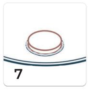
Carefully push extra silicone around any gaps between drain and sink, as needed.
