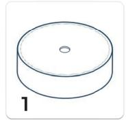
Run a **generous** amount of clear silicone around the underside of the basin 1" back from the outer edge.
