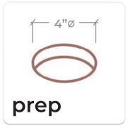
Cut large enough opening in surface (4" diameter) for plumbing to attach to basin **only**.
