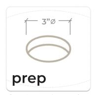
Determine exact placement of basin on the surface. Reference footprint dimensions (right). Cut exactly a 3"diameter opening in surface.
