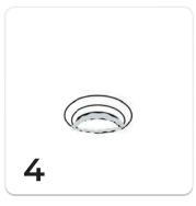
Run a **generous** amount of clear silicone around the drain rim. It is important that the silicone overflows when drain is placed through the opening.
