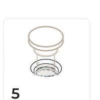
Slide drain into place and add a **generous** amount of silicone to drain seal or nut underneath. Secure drain by hand tightening no more than a ½" turn. **Do not overtighten.**
