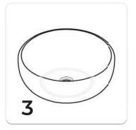
Run a bead of clear silicone to fill the gap between the underside of basin and the surface. Smooth silicone off to a neat finish. Ensure edge is fully waterproofed. Allow silicone to sit and dry for 12 hours prior to installing plumbing fixtures in step 4, 5 and 6.
