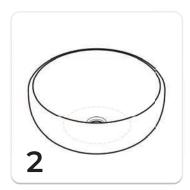
Flip and press down onto the surface. Be mindful of the basin base to ensure it is **centered around the surface opening**. A template may assist with the basin's placement. Remove excess silicone and wipe clean with a microfiber cloth.
