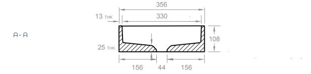
mudd works to tolerances of +/- 5mm. SCALE 1:8 2/2
